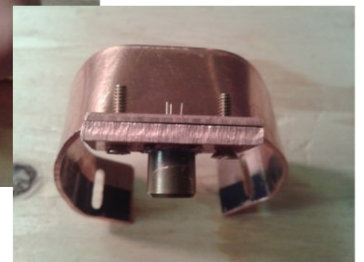
1st & 2nd heat sink prototype for laser above
